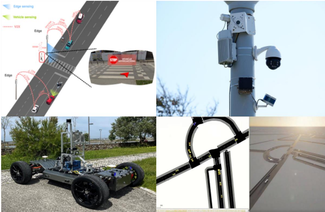
Figure 57. Scenario to detect potential collisions (top left); ATCLL smartlamp post (top right); Autonomous vehicle development platform (bottom left); and ATCLL digital twin application (bottom right)
